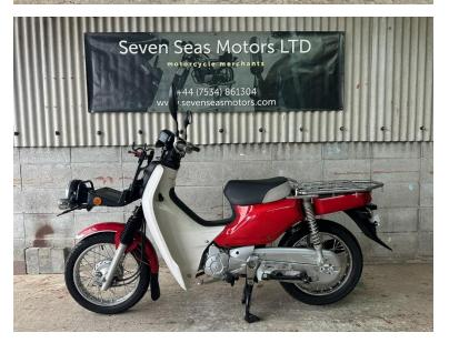
You can tell the C110 Pros were used for commercial use by the way the headlight is fitted below the rack. This way, no matter how much you're carrying, your headlight will still light up the road in front.
